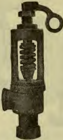
FIG. 384.—A pop safety valve designed especially for use with superheated steam. The spring, as is shown in the figure, is not enclosed and is therefore protected from the high temperature of the steam. This is necessary as intense heat soon takes the temper out of the spring and destroys its elastic properties.
